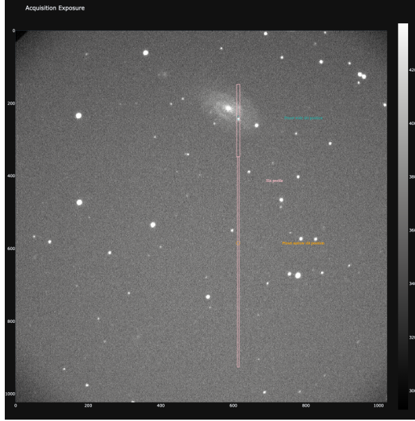
Fig. 6. Presented is the acquisition image from the rapid spectroscopic follow-up of SN 2023yoo using Mookodi. The robotic system utilizes Mookodi in imaging mode, coupled with astrometric calibration to precisely and automated position the requested RA and DEC within the appropriate section of the spectrograph’s slit. In this instance, RA=22:01:03.150 and DEC=-13:16:28.99, and the request specified the use of the “wide slit” (depicted by the pink outline, illustrating the location of Mookodi’s stepped-slit, with a \sim 6 -arcmin-long “narrow slit” of 2 arcseconds and \sim 2 -arcmin-long “wide slit” of 4 arcseconds). The resulting spectrum can be viewed on the Transient Name Server (TNS) at: https://www.wis-tns.org/object/2023yoo .
