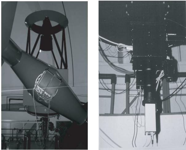
Fig. 1. The 1.52-m telescope and the speckle camera attached to it.
