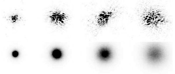
Fig. 1. Examples of speckle patterns generated using the Random Wave Vector algorithm. Above : examples of single frames, Below : average of 1000 images (long exposure outcome). From the left : D/r_0 = 1, 3, 5 and 7 .
