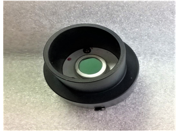
Figure 1. MIR detector module. (a) Schematic of detector integration into the chassis. (b) Prototype of the MIR detector module in an anodized aluminum chassis. The chassis had a standard diameter of 1.25-inch in. The MIR detector module can be installed in the place occupied by a conventional eyepiece, facilitating its coupling to a commercial telescope.
