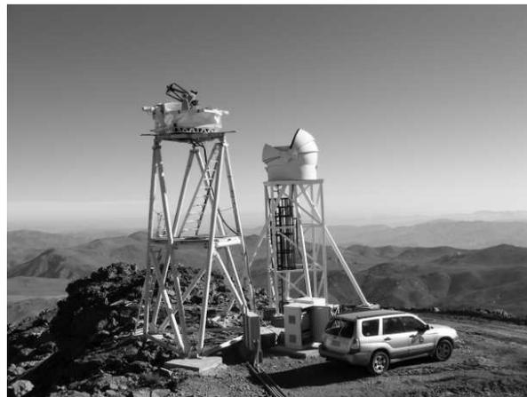
Fig. 2. The Peñon site with the two site monitoring telescopes on their respective towers, and with their domes opened. To the left (South) the TMT-T1 site testing telescope, to the right (North) the LSST one. Photograph courtesy CTIO site team.
