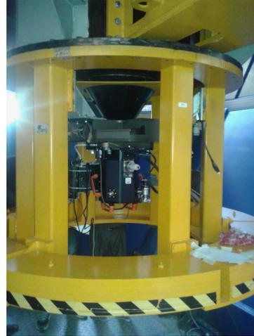
Fig. 3. The fully assembled 4K×4K CCD camera along with shutter and automated filter wheels mounted at the axial port of the 3.6m DOT on 9th December 2015.
