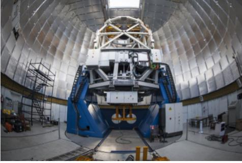
Fig. 1. The 3.6m DOT as installed at Devasthal Nainital by a Belgian company AMOS (fall 2015) inside the dome build indigenous by an Indian firm. This telescope is installed at nearly 11-m height from the ground level to improve seeing.
