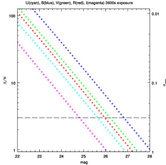
Fig. 2. A simulated plot of magnitude (X-axis) vs. signal-to-noise ratio (Y-axis, left) and corresponding error in the magnitude determinations (Y-axis, right) based on the throughput calculations (Mayya 1991) of the 3.6m telescope with the proposed 15 micron 4K×4K CCD camera for set of Bessel *UBVRI* filters, for assumed equivalent exposure time of 1 hour each, seeing value of 1.5 arc-sec. and for other standard values of the observing site and the CCD chip (STA 15-micron).
