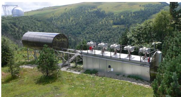
Fig. 2. Photo of the all 9 channels of MMT installed on 5 mounts in the single cylindrical dome, which is open at that moment. The russian 6-m telescope may be seen in the background.
