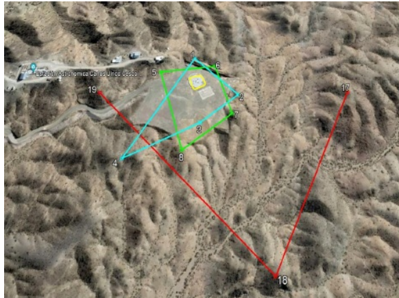
Figure 2. Internal, intermediate and external networks for CART foundation monitoring.
