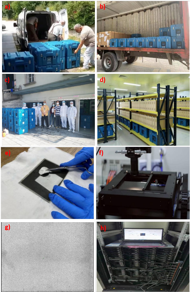
Figure 3. The entire process photographic plates preservation. a) packaging and transporting (in that case from Uzbekistan). b-c) Reception in Shanghai. d)Storage in an archive room at controlled temperature and humidity. e) Cleaning of the plate. f-g) Digitization. h) Saving in digital form in a dedicated server.
