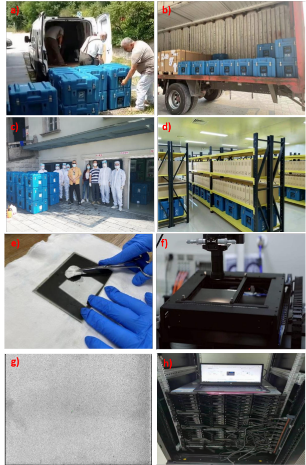
Fig. 3. The entire process photographic plates preservation. a) packaging and transporting (in that case from Uzbekistan). b-c) Reception in Shanghai. d) Storage in an archive room at controlled temperature and humidity. e) Cleaning of the plate. f-g) Digitization. h) Saving in digital form in a dedicated server.
