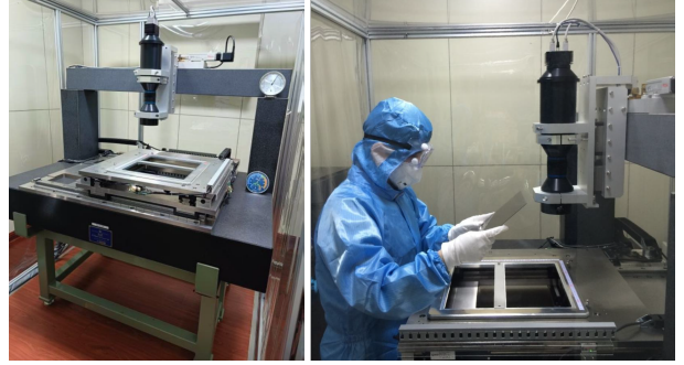
Fig. 1. First high-precision astronomical plate digitizer based on mechanical guide rails.
